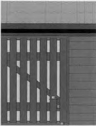
Shutter shutter detail to existing opening. Closed screen behind, inward opening to allow for cleaning 1:10
